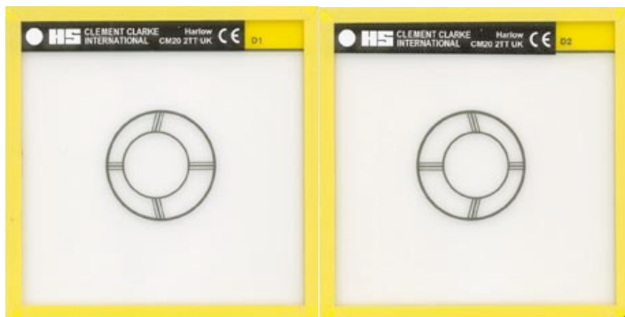
Figure 3. 3rd-degree fusion slides: Common fusible images with a slight offset in some features to create disparity and stimulate stereopsis.
