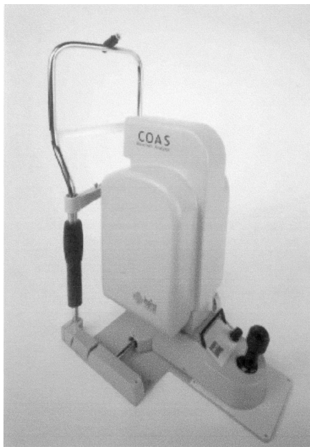
FIGURE 1. The current version of the Complete Ophthalmic Analysis Systems (COAS). It is similar to an autorefractor in size and operation.
